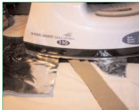
Figure 2. Care must be taken to avoid getting the iron-on tape glue on areas of the splint that will receive the Velcro hook. This glue impedes the hook and neoprene plush bond. Protect the plush material with foil when ironing the tape in place.
